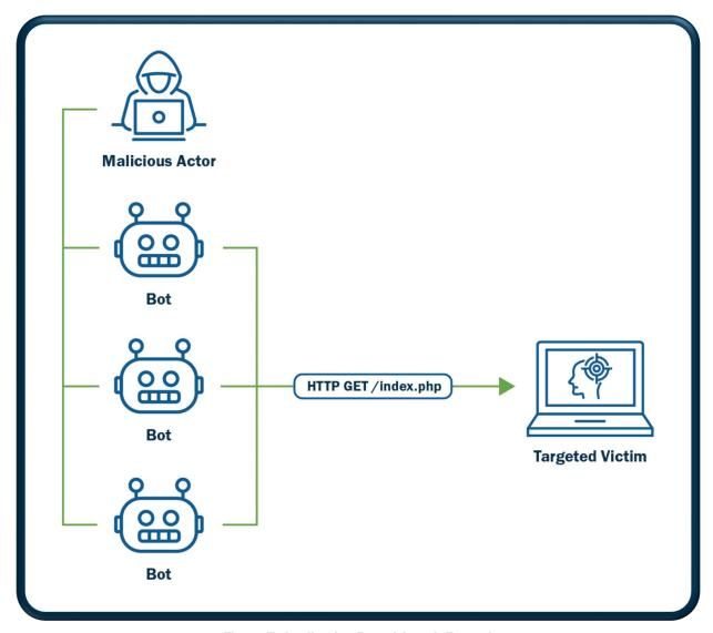
Figure 7: Application-Based Attack Example
