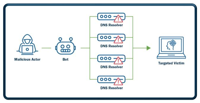
Figure 3: Volumetric-Based Attack Example
